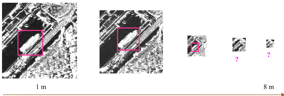
Figure 16: Retrieved information for a set of five patches in the port having a resolution from 1 m to 8 m. Trying to identify an object from 1m to 8m, for example the ship, we can notice that for the last two resolutions this is not possible anymore.
